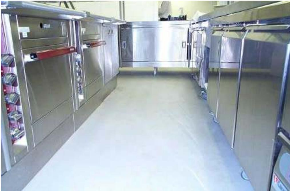
[Ryegrip Quartz](#) 4-6mm decorative heavy duty anti-slip epoxy resin floor screed.
