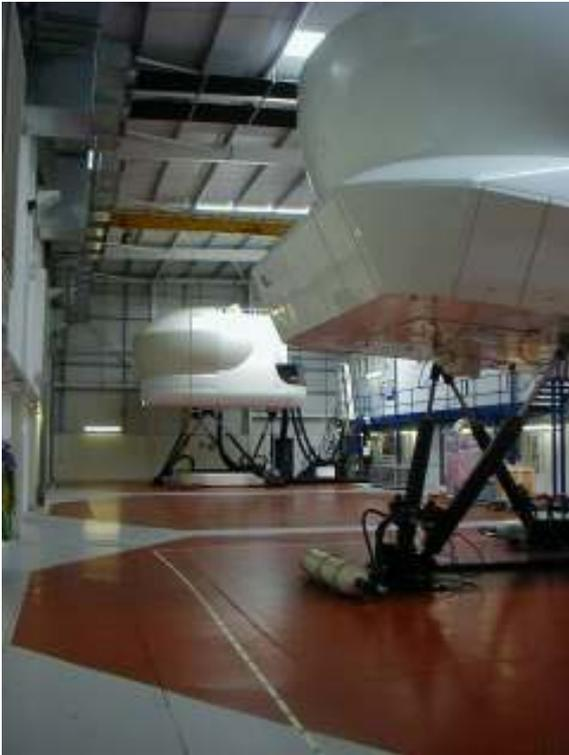
Weighing thousands of kilograms, the four flight simulators at Alteon Training near Gatwick, require a 1½ metre thick concrete base for support. Avoiding the final floor finish delaminating due to the high moisture level inherent in such a substantial concrete base, Ryebrook Resins recommended their water-dispersed, Ryecoat WD epoxy coating.
